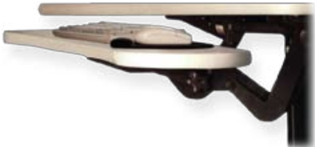
{ F } EasyMate™ Item No. 294XX xx = 15 for 15 lb spring assist xx = 20 for 20 lb spring assist Travel range: 6" up, 6" down +9° to -15° tilt Lift and Set, spring- assisted height positioning Not retractable Numerous widths available Steel, Black Powder Coat
