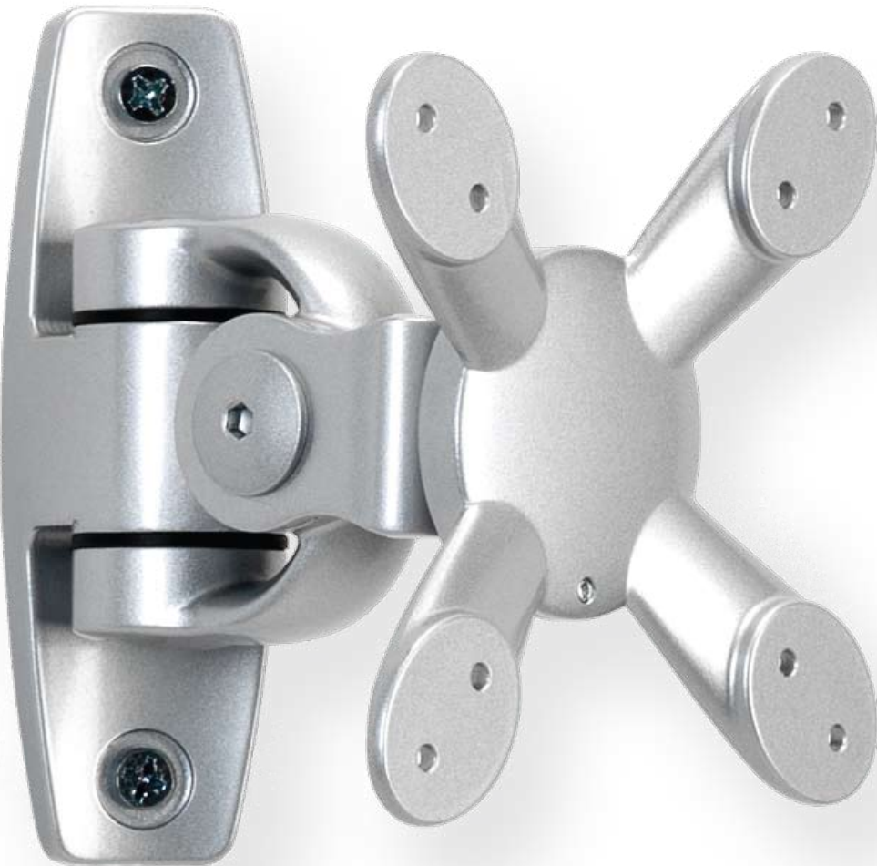
{C} Super Stubby EasyWall Monitor Arm Item No. 28653 Tilt +/- 100° Swivel Limited Rotation +/- 180° Monitor Capacity 33 lbs Material Aluminum Alloy Finish Silver Powder Coat
