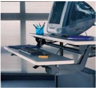
{ G } PositionMate™ Item No. 187XX xx = 15 for 15 lb spring assist xx = 20 for 20 lb spring assist Travel range: 7" up, 5.75" down +9° to -15° tilt Paddle-actuated height positioning Not retractable Numerous widths available Steel, Black Powder Coat
