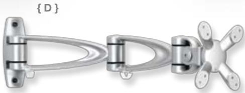
{D} EasyWall Monitor Arm Item No. 28651 Forward Reach 4" to 17" Tilt +/- 100° Swivel +/- 90° Rotation +/- 180° Monitor Capacity 33 lbs Material Aluminum Alloy Finish Silver Powder Coat
